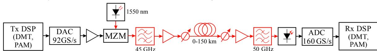
Figure 1. Optical setup for an intra-cluster connection. The link length is varied between 0 km and 150 km.
