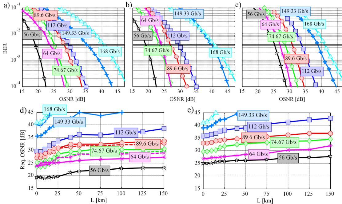
Figure 3. Simulation results. Back-to-back performance for: a) TDH-PAM, b) multidimensional modulation and c) DMT. The HD-FEC limit ( $BER = 3.8e-3$ ) is marked as a reference. The OOK, PAM-4 and PAM-8 curves are also included in a) and b). The required OSNR for the HD-FEC limit at varying fiber lengths is depicted in d) for TDH-PAM and multidimensional modulation (dashed curves) and in e) for the DMT setup.
