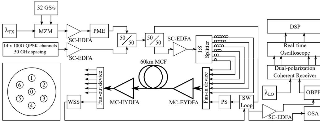
Fig. 2: System setup and core identifiers for the MCF.
