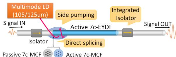
Fig. 1: Schematic of the internal structure of the MC-EYDFA.
