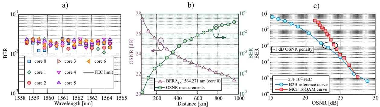
Fig. 3: a) BER measurements for the 200 Gbit/s 16QAM channel with 14 x 100 Gbit/s QPSK neighboring channels after 720 km. b) OSNR (left y-axis) and BER (right y-axis) measurements for the TC at a wavelength of 1564.271 nm for different transmission distances. c) BER vs. OSNR comparison between optical B2B and the corresponding BER-OSNR points presented in Fig. 3 (b).
