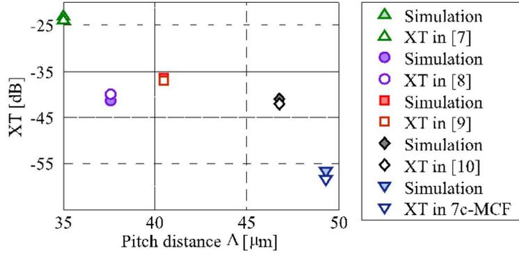
Figure 3. Comparison between measured XT in manufactured MCFs in the literature and XT estimations from MCF modelling from FEM and PCT.
