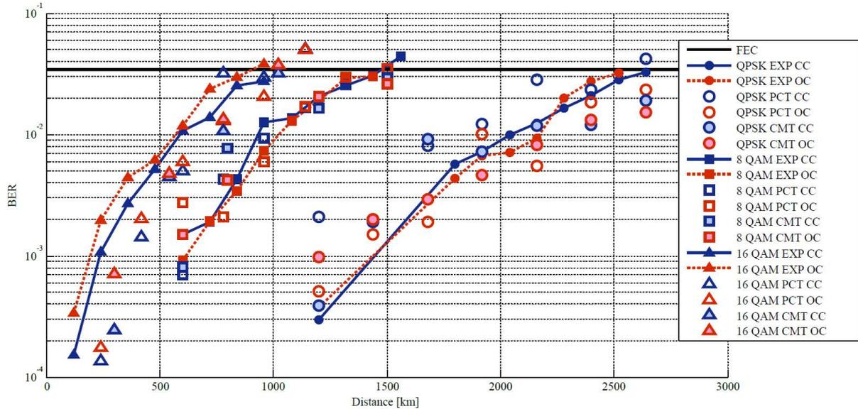
Figure 5. Comparison between experimental transmission results and simulation results from CMT and PCT.
