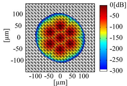
Figure 2. Cross-sectional view of the normalized power distribution in a 7-core MCF.
