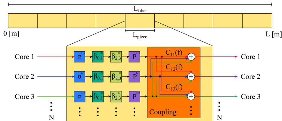
Figure 1. Fiber structure for a simulation model of an MCF.
