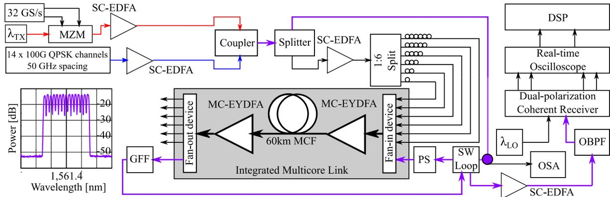
Figure 4. Experimental setup of a 7-core MCF system with an integrated multicore link.
