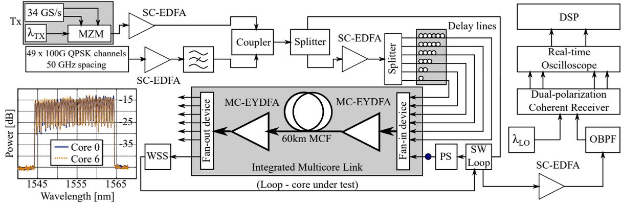
**Fig. 2:** Experimental setup and spectra of the inner core and one outer core before the integrated multicore link. ( $\lambda_{TX}$ : transmitted wavelength for the channel under test,  $\lambda_{LO}$ : wavelength for the local oscillator)
