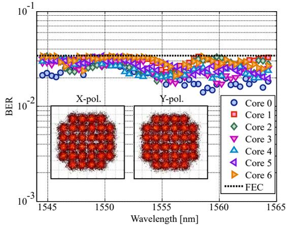
**Fig. 3:** BER measurements after 180 km using a recirculating loop and an IML for the 32-QAM channel at different wavelengths. As insets, the constellation diagrams for a BER value of  $3.4 \cdot 10^{-2}$  are shown.
