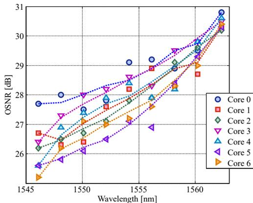
**Fig. 4:** OSNR measurements for all seven cores of the MCF. Figure 4 displays the OSNR measurements after 180 km for 9 uniformly spaced channels between 1546 nm and 1562 nm. OSNR readings match the observations extracted from Fig. 3, confirming that the cores with the lowest OSNR
