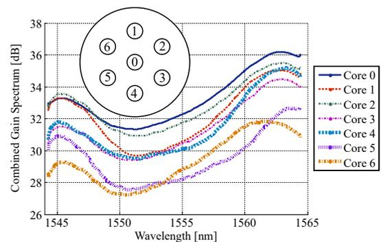
**Fig. 1:** Structure of the MCF and cascaded gain spectrum of both MC-EYDFAs for one loop iteration corresponding to pump currents of 3.0 A and 2.2 A (loss caused by the fiber and fan-in/fan-out couplers is neglected).
