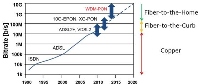
Fig. 2: Comparison of different access network technologies [3]
