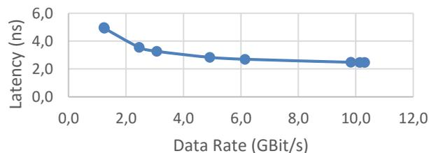
Fig. 4: Latency measurement at the low-latency cross-connect
