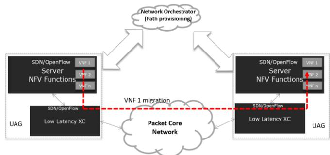
Fig. 6: VNF migration over temporary provisioned path by SDN network orchestrator
