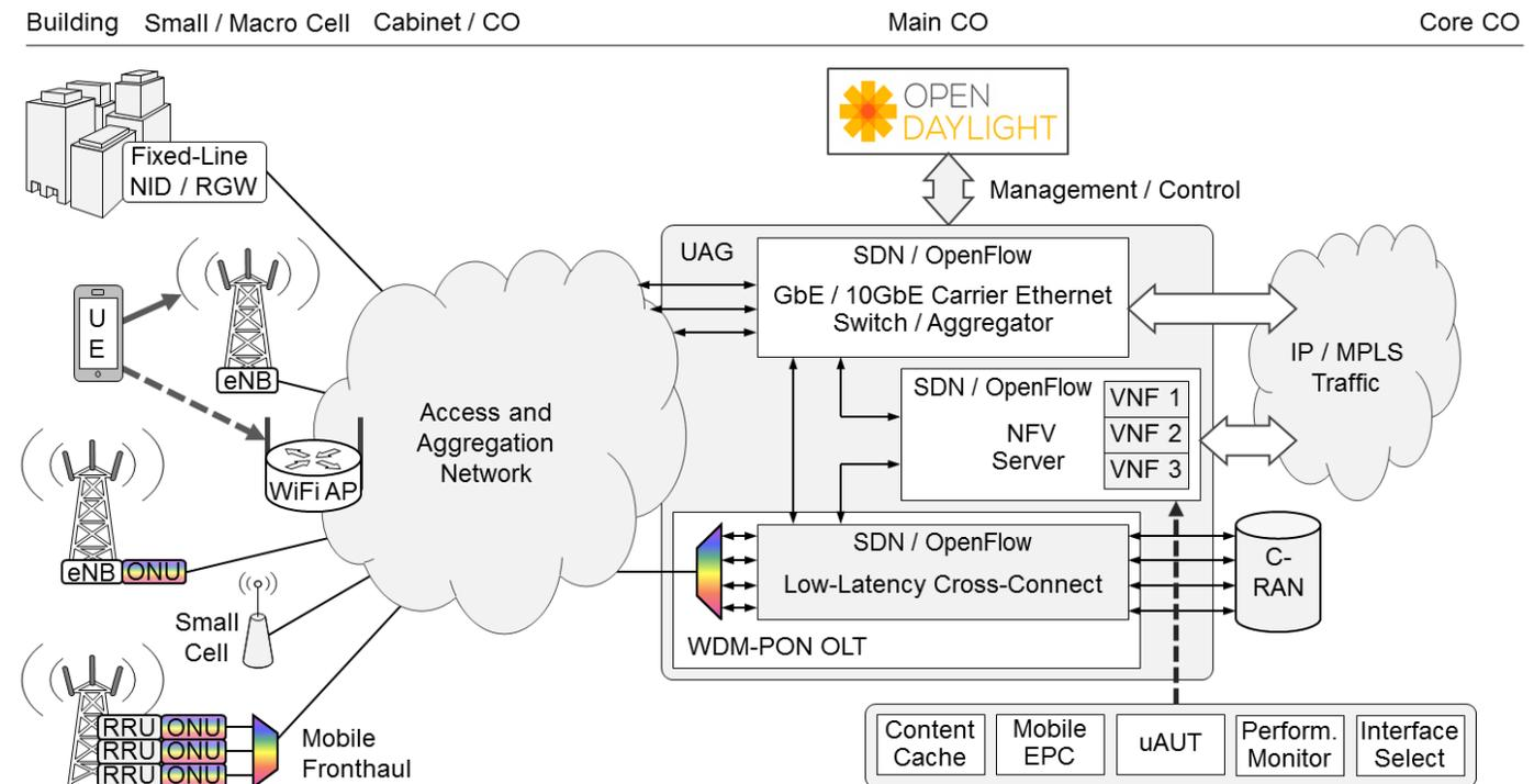
**Fig. 3:** FMC system architecture. (NID: network interface device; RGW: routing gateway; UE: user equipment; ONU: optical network unit; RRU: remote radio unit; UAG: universal access gateway; OLT: optical line terminal; VNF: virtual network function; EPC: evolved packet core; uAUT: universal authentication)
