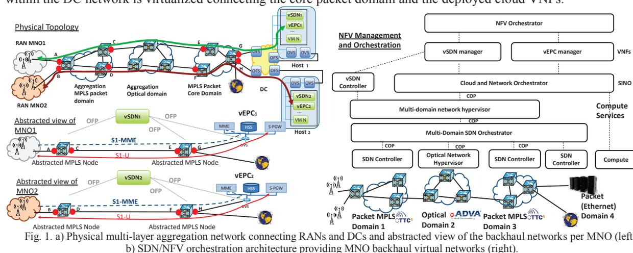
Fig. 1. a) Physical multi-layer aggregation network connecting RANs and DCs and abstracted view of the backhaul networks per MNO (left). b) SDN/NFV orchestration architecture providing MNO backhaul virtual networks (right).
