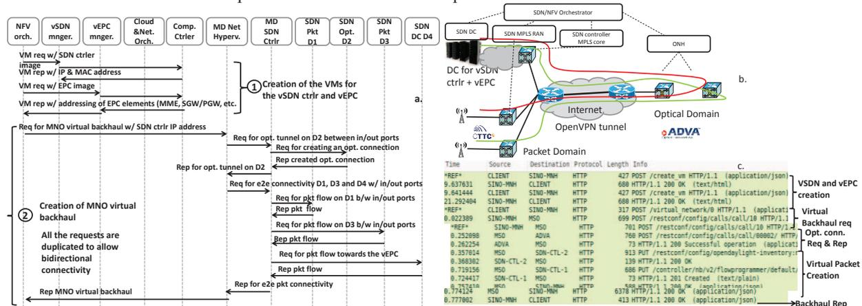
Fig. 2. a) Workflow for provisioning MNO virtual backhaul network and VNFs. b) Topology of the connectivity between CTTC SDN/NFV Orchestrator and the ADVA ONH. c) Capture of the experimental control messages for setting the VNFs and virtual backhaul network.
