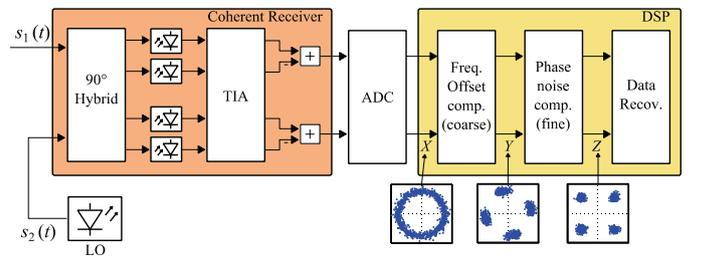
Fig. 6. Intradyne detection based on QPSK-DSP
