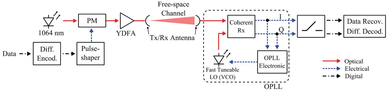
Fig. 2. Homodyne Detection setup of a state-of-the-art optical intersatellite communication system
