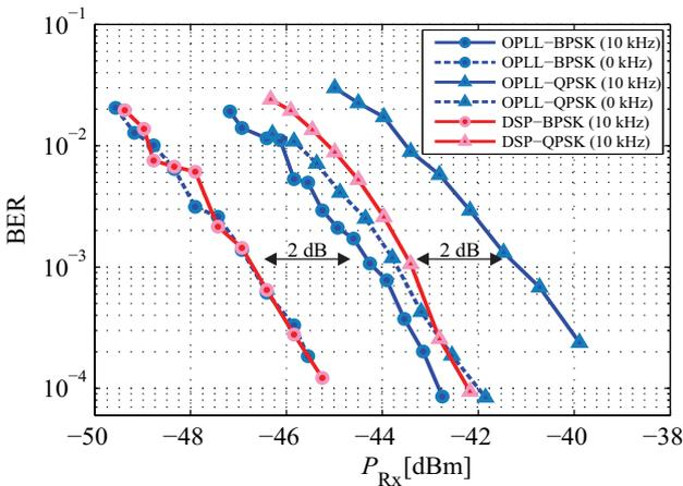
Fig. 9. BER vs. received input power in OISL; comparison of the two detection schemes for BPSK and OPSK
