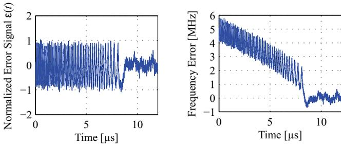
Fig. 4. Lock-in process: phase error (left) and frequency error (right)
