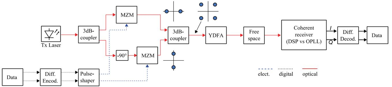
Fig. 8. Block diagram of the QPSK simulation setup
