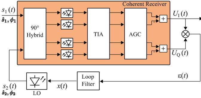
Fig. 3. Optical phase-locked loop based on Costas-loop implementation
