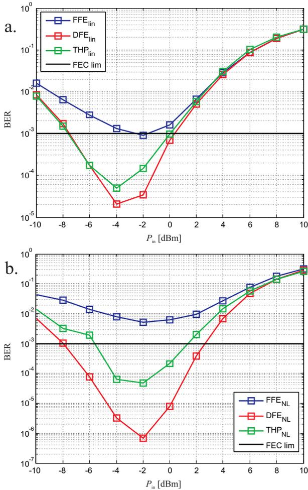
**Figure 5** BER vs. launch power for 500 km transmission in case of a. linear equalization and b. VNLE.
