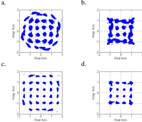
**Figure 4** Equalized constellation diagrams for THP: a. THP(1)-FFE(3) before modulo decoding, b. THP(1)-FFE(3) after decoding, c. THP(1)-VNLE(3) before modulo decoding, d. THP(1)-VNLE(3) after decoding.
