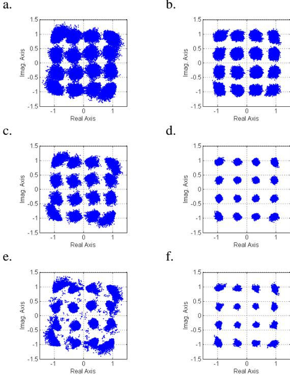
**Figure 3** Equalized constellation diagrams: a. FFE(3), b. VNLE(3), c. FFE(4), d. VNLE(4), e. FFE(3)-DFE(1), f. VNLE(3)-DFE(1).
