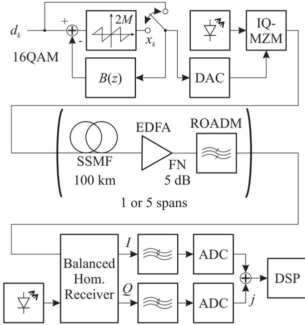
Figure 1 System setup
