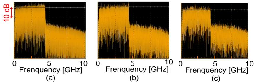
Fig. 2: Spectra (measured at the DSO) with power loading of (a) optical B2B signal, (b) center launching signal, (c) offset launching signal.
