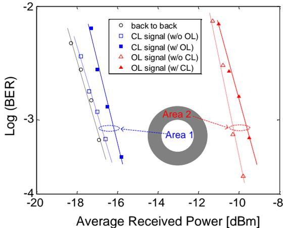
Fig. 3: BER measurement results. **CL**: center launching, **OL**: offset launching.
