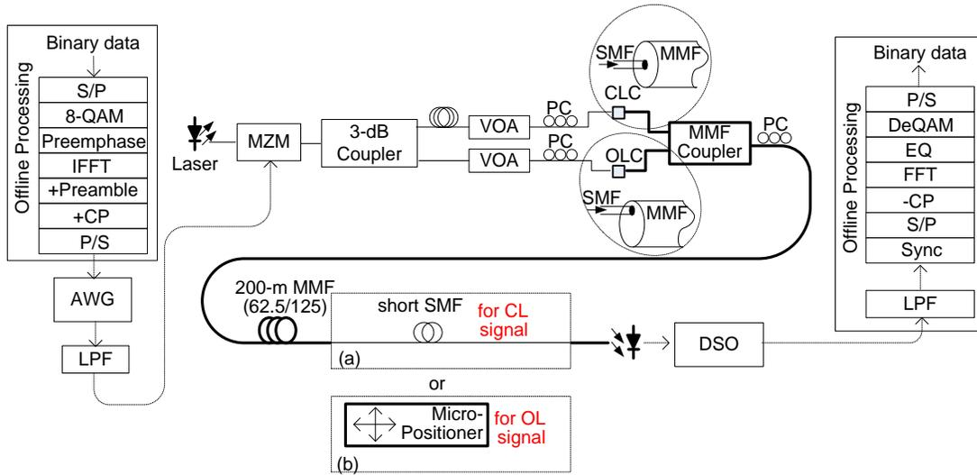
Fig. 1: Experimental setup of the 25.5-Gb/s  $2 \times 2$  OFDM-MGDM transmission over a 200-m OM1 MMF. **CL**: center launching, **OL**: offset launching.
