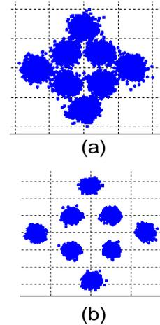
Fig. 4: Constellation of (a) offset launching signal, (b) center launching signal.
