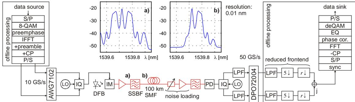
Fig.2: Experimental DS setup with one OLT and one ONU with digitally reduced sample rate and reduced DSP complexity by a factor of  $r$
