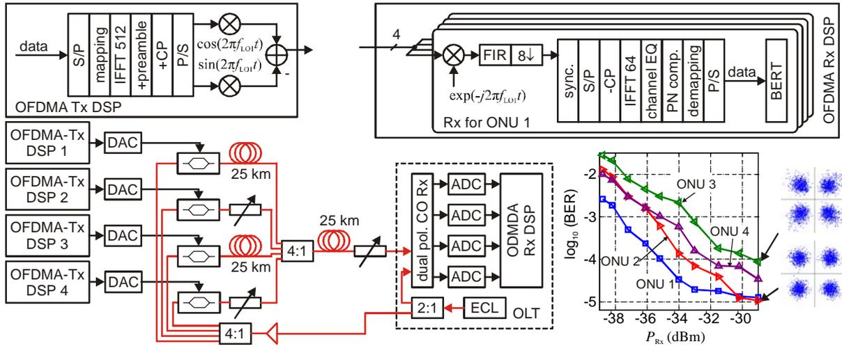
Fig. 4. Experimental US setup with four transmitting ONUs and coherently receiving OLT.
