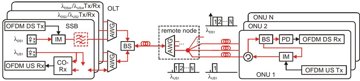
Fig. 1. Proposed architecture of the OFDMA-PON (US=upstream, DS=downstream, BS=band splitter, IM=intensity modulator).
