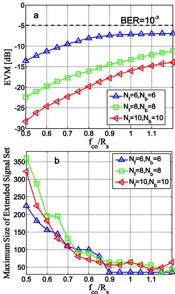
Figure 7 Effect of the receiver filter on the performance of THP: (a) EVM and (b) maximum number of symbols in the extended signal set vs. the normalized cut-off frequency of the receiver filter.
