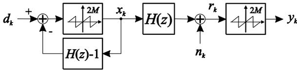
**Figure 2** A communication system with THP.
