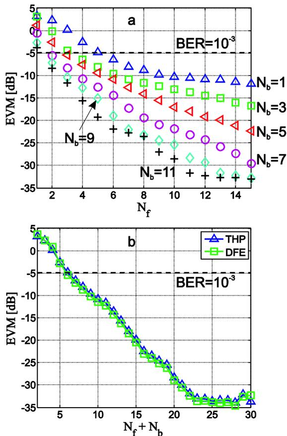
**Figure 8** Compensators performance for a varying number of filter coefficients: (a) EVM vs.  $N_f$  for six different  $N_b$  values in case of THP (b) optimal EVM for a restricted total number of filter coefficients  $N_f + N_b$ .
