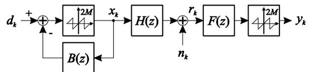
**Figure 5** A communication system with THP and an FFE for effective compensation of pre- and post-cursor ISI.
