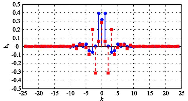
**Figure 4** Real (blue circle) and imaginary (red square) components of a sampled impulse response of a system with a raised-cosine-in-time-domain pulse shaping filter and 400 km of SSMF
