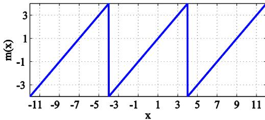
**Figure 3** A zero-mean  $2M$  modulo function for a 4-ASK modulation format ( $M=4$ ).
