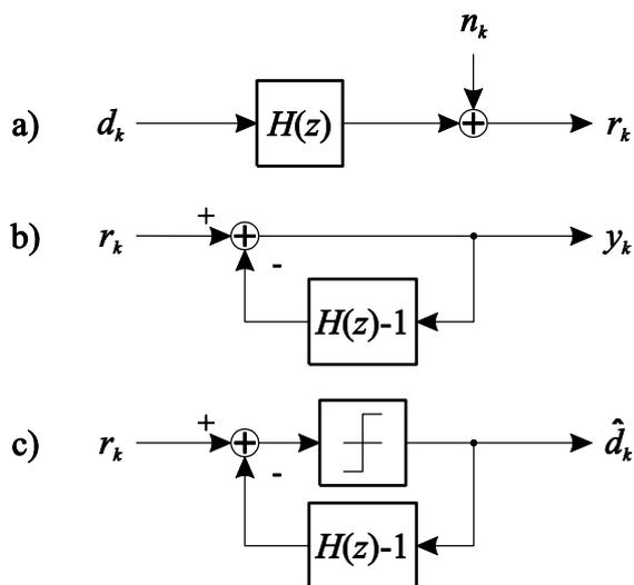
**Figure 1** Discrete-time models of (a) an ISI-AWGN channel, (b) a zero-forcing IIR equalizer and (c) a decision-feedback equalizer.
