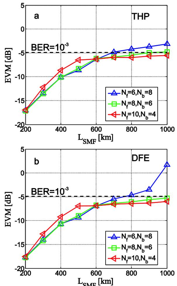
**Figure 9** Compensators performance for a varying transmission length: EVM vs. the length of the transmission link in case of (a) THP and (b) DFE.
