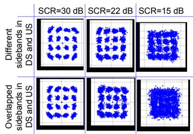
Fig. 3: Upstream constellations under different SCR levels.
