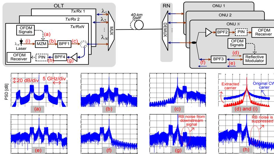
Fig. 1: Proposed lightwave centralized WDM-PON architecture using upper and lower sideband OFDM signal in downstream and upstream, respectively. Insets (a)-(h): simulated power spectral density (PSD) corresponding to point (a)-(h) marked in the architecture.
