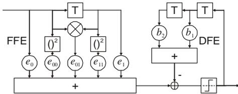
Fig.4. Example of nonlinear Volterra equalizer with nonlinear feed forward and linear decision feedback part
