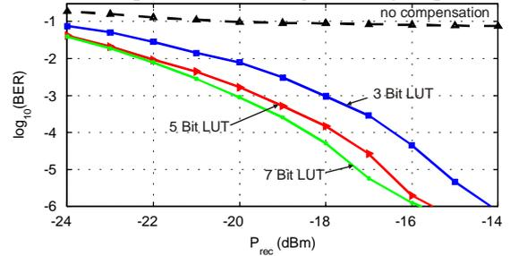
Fig.5. BER vs. received optical power with pre-compensation
