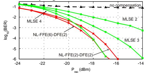
Fig.6 BER vs. received optical power with post-compensation
