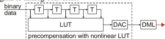
Fig.2. Efficient implementation of pre-compensation of the laser current
