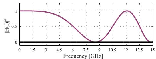
Fig. 1: Power fading described by the frequency response function in a dispersive channel between a frequency of 0 and 15 GHz for a 50 km SSMF ( $D = 17$  ps/nm/km)
