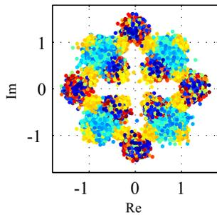
Fig. 8: Received constellation at increased bit rate of 15.9 GBit/s, 720 used subcarriers modulated with QPSK, 8-QAM and 16-QAM and SSB transmission
