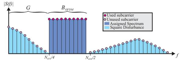
Fig. 3: OFDM bandwidth allocation with direct detection and MZM
