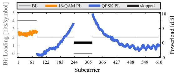
Fig. 5: BL and PL scheme for 610 used subcarriers for DSB transmission
