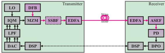
Fig. 4: Simplified measurement setup for a 50 km PON scenario with optional single sideband filter (dashed)
