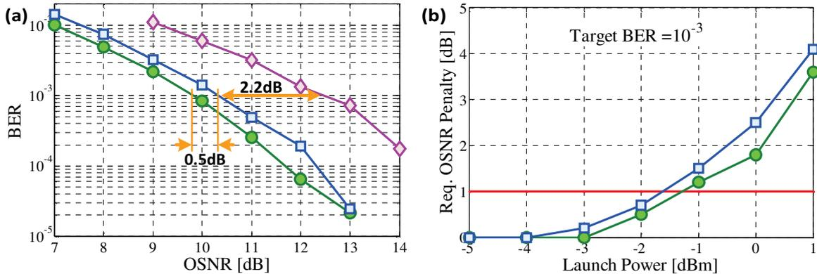
**Fig.3:** (a) BER as a function of OSNR for back-to-back scenario for  $\square$  ILL-OFDM at ILL Input Power = -37dBm, CSR = -4dB,  $\bullet$  CO-OFDM at CSR = -10.2dB and  $\blacklozenge$  SCO-OFDM at CSR = -5.4dB
