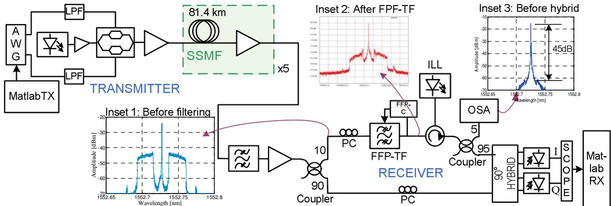
**Fig. 1:** Schematic of injection locked laser based self coherent optical OFDM system with Inset 1: optical spectrum before carrier extraction, Inset 2: optical spectrum after FPF-TF and Inset 3: optical spectrum after carrier extraction; FP-TF/C: Fabry-Perot tunable filter/controller, PC: polarization controller, ILL: injection locked laser, OSA: optical spectrum analyzer.
