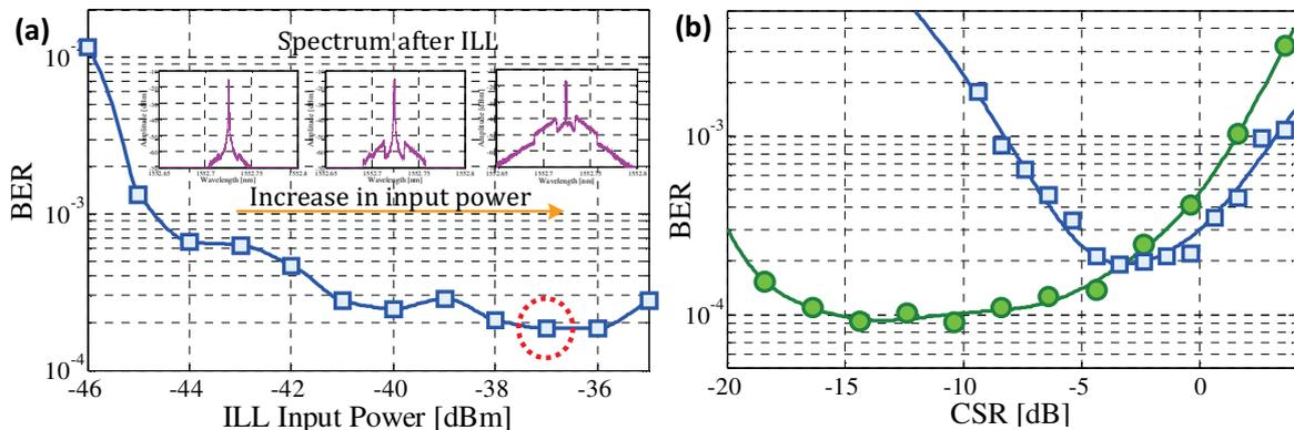
**Fig. 2:** BER curves at a required OSNR of 12dB (a) as a function of ILL input power with CSR = -4dB, (b) as a function of CSR for  $\square$  ILL-OFDM with ILL Input Power = -37dBm and  $\bullet$  CO-OFDM
