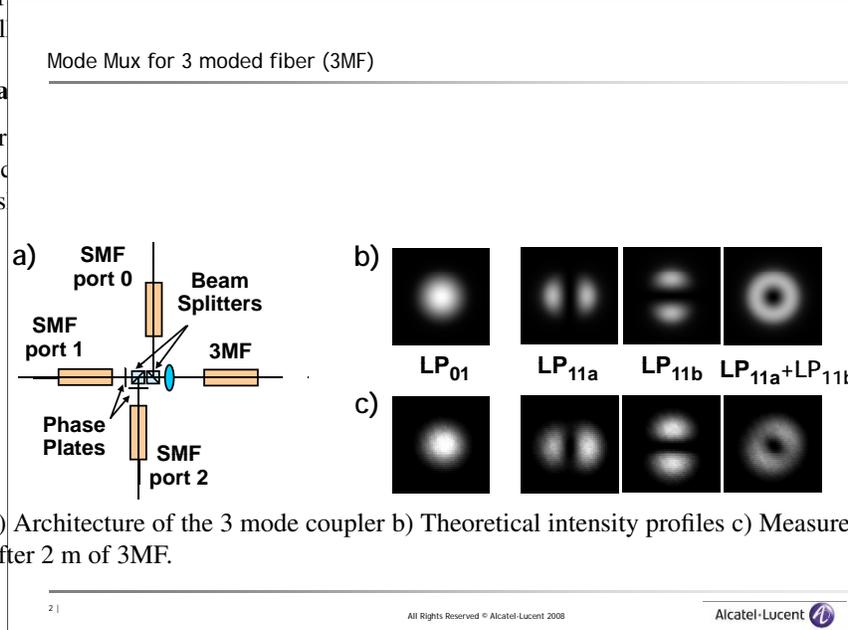
Fig. 1. a) Architecture of the 3 mode coupler b) Theoretical intensity profiles c) Measured intensity profile after 2 m of 3MF.
