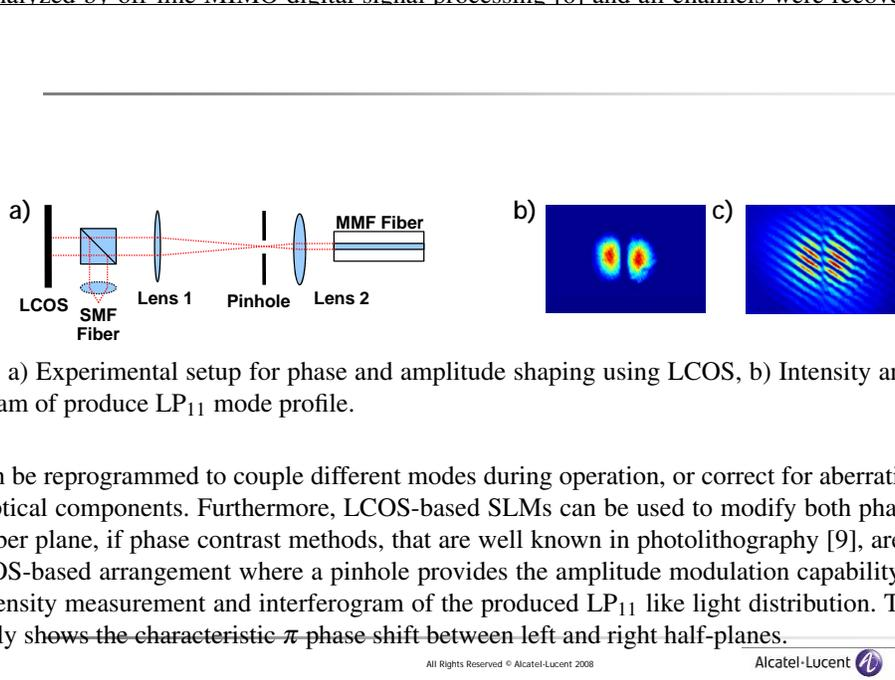
Fig. 3. a) Experimental setup for phase and amplitude shaping using LCOS, b) Intensity and Interferogram of produce LP<sub>11</sub> mode profile.
