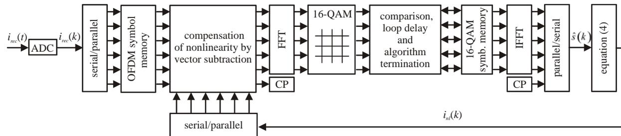
Fig. 1. Block diagram of proposed method for compensation of nonlinearity in the receiver.
