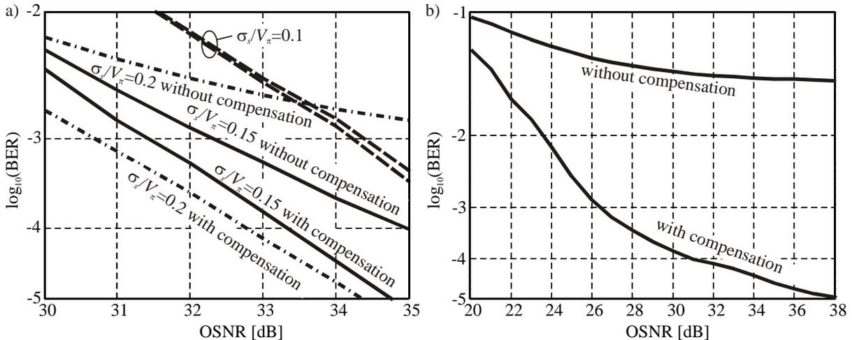
Fig. 2 a) BER vs. OSNR (measured within 0.1 nm bandwidth) for quadrature bias; b) BER vs. OSNR for  $V_{\text{bias}} = -0.8V_{\pi}$  and  $\sigma_s = 0.1V_{\pi}$ .
