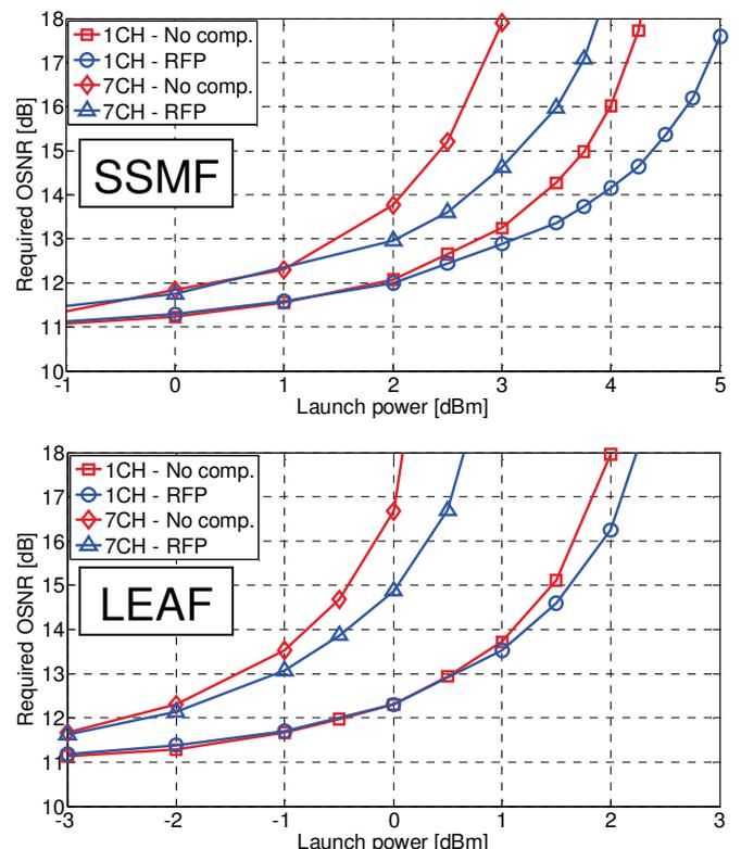
Fig. 4: Required OSNR for a BER of  $10^{-3}$  as a function of the launch power.
