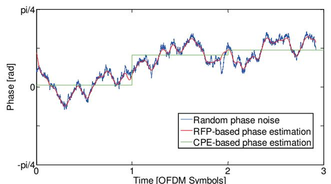
Fig. 2: Example of random phase noise evolution over three OFDM symbols together with results of CPE estimation and RFP phase noise estimation.
