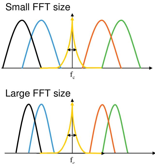
Fig. 3: Illustration of RFP with small and large FFT size
