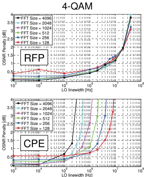
Fig. 1: Phase noise tolerance for RFP and CPE with varying FFT size.
