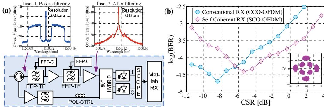
**Fig. 1:** (a) Schematic of self coherent optical (SCO-) OFDM system with Inset 1: optical spectrum before FFP-TF series and Inset 2: optical spectrum after FFP-TF series; FFP-TF/C: fiber Fabry-Perot-tunable filter/controller, (b) BER as a function of CSR.
