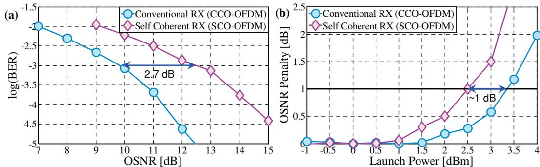
**Fig. 2:** (a) BER as a function of OSNR for back-to-back scenario, (b) Required OSNR penalty as a function of the launch power after 400km transmission.
