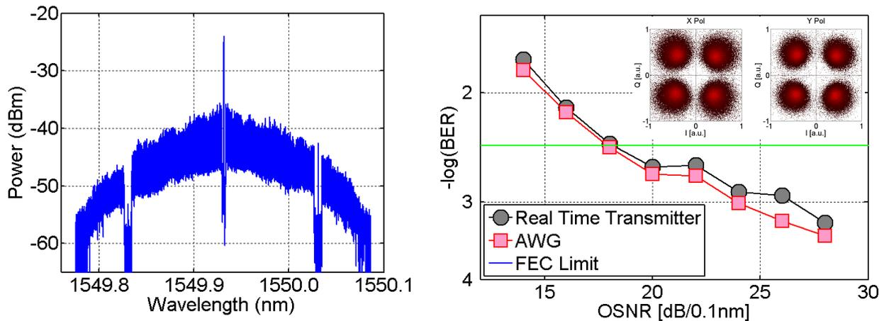
Fig. 2a: Optical spectrum of the 93.8-Gb/s OFDM signal, Fig. 2b: BER performance as a function of the OSNR (inset: constellation diagram of both polarizations at high OSNR).
