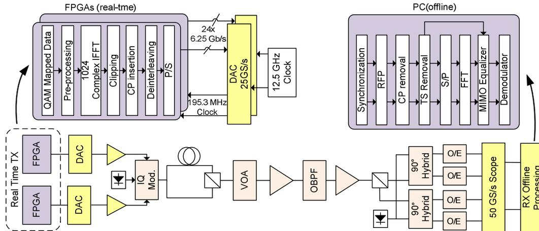
Fig. 1: Experimental setup including real time transmitter with FPGA and DAC boards, optical setup and offline processing blocks.
