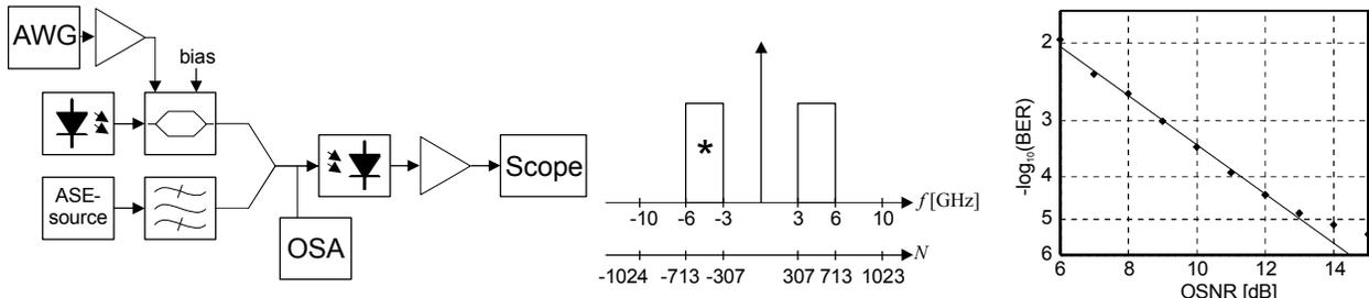
Fig.1. Experimental setup (left), OFDM subcarrier allocation (center), and BER result (right) for 6 Gb/s DD-OFDM b2b measurement.
