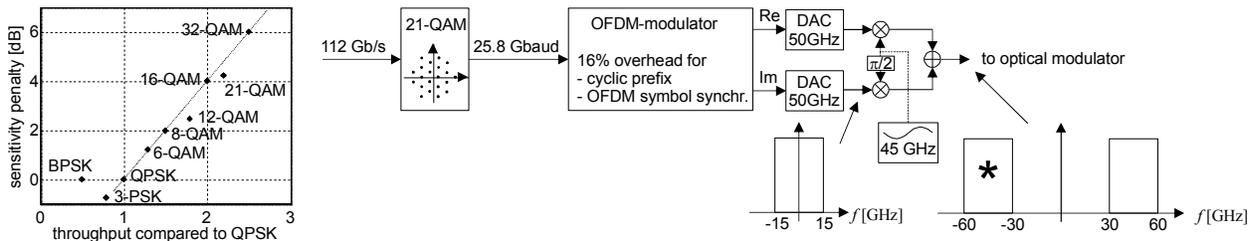
Fig. 2. Sensitivity penalty for several digital modulation formats (left), and block diagram for generation of OFDM modulator signal with 60 GHz bandwidth containing 100 Gb/s net data rate using 21-QAM digital modulation.
