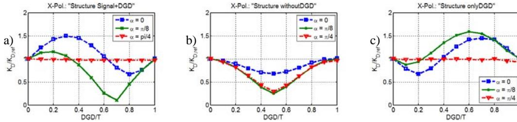
Fig. 3:  $K_D/K_{D,ref}$  vs. DGD/T ( $K_{D,ref}$  is the  $K_D$  at DGD = 0T and  $\alpha = 0$ ) for various polarization mixing angles  $\alpha$  for a) "Structure Signal+DGD", b) "Structure withoutDGD" and c) "Structure onlyDGD"
