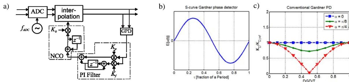
Fig. 1: a) Fully digital clock recovery, b) S-curve of the Gardner phase detector and c) normalized phase detector constant vs. DGD/T for various polarization mixing angles  $\alpha$  for clock recovery with conventional Gardner PD.
