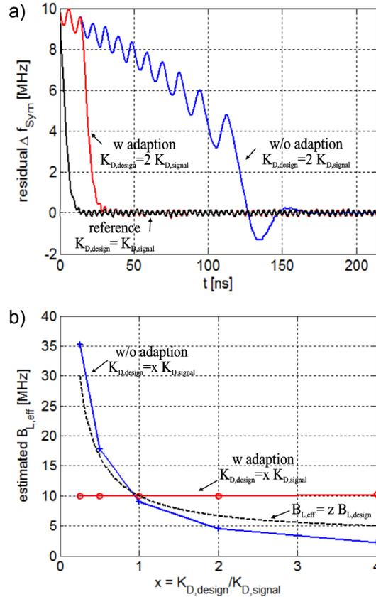
**Fig. 3:** a) Residual  $\Delta f_{\text{Sym}}$  during the lock-in procedure for a system with and without adaptive control with  $K_{D,\text{design}} = 2 K_{D,\text{signal}}$  and a reference system with  $K_{D,\text{design}} = K_{D,\text{signal}}$  and b) estimated loop bandwidth  $B_{L,\text{eff}}$  after PI-filter for both systems and  $B_{L,\text{eff}} = z B_{L,\text{design}}$  (equation (2) and (3)) vs.  $x$  after lock-in of the PLL
