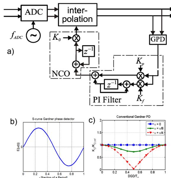
**Fig. 1:** a) Fully digital clock recovery, b) S-curve of the Gardner phase detector and c) normalized phase detector constant vs.  $DGD/T_S$  for various polarization mixing angles  $\alpha$  for clock recovery with conventional Gardner PD.
