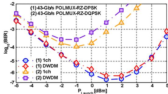
**Fig. 4:** Launch power vs. BER after 5700km of SSMF (Simulation)
