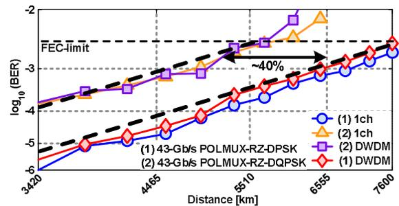
**Fig. 5:** Distance vs. BER with optimal launch power (Experimental)
