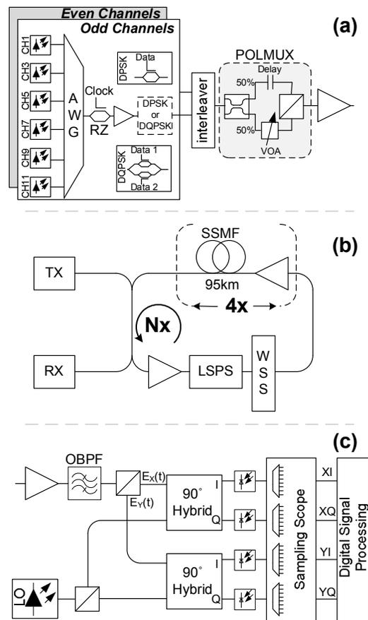
**Fig. 1:** Experimental Setup, (a) Transmitter, (b) Recirculating loop and (c) Coherent receiver
