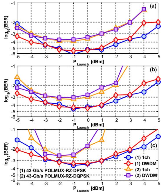
Fig. 3: Launch power vs. BER after (a) 3420km, (b) 4560km and (c) 5700km of SSMF (Experimental)
