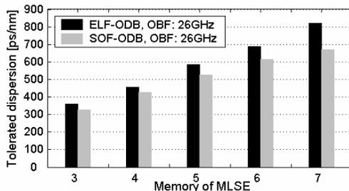
Figure.4: Tolerated dispersion for ELF-ODB and SOF-ODB by using an MLSE with different memories at an OSNR of 18dB to achieve BER=5x10<sup>-4</sup>.
