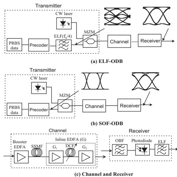
Figure.1 system setups, (a) ELF-ODB, (b) SOF-ODB, (c) the channel and receiver.
