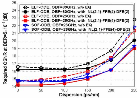
Figure.2 Required OSNR at BER=5x10<sup>-4</sup> versus the dispersion for ELF-ODB and SOF-ODB with and without using NL(2,1)-FFE(4)-DFE(2).
