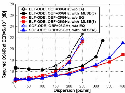
Figure.3 Required OSNR at BER=5x10<sup>-4</sup> versus the dispersion for ELF-ODB and SOF-ODB with and without using MLSE(3).
