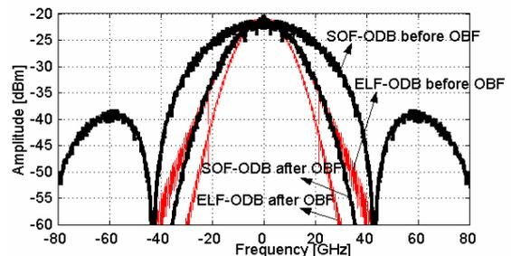
Figure.5: Spectra of SOF-ODB and ELF-ODB before and after optical filtering.
