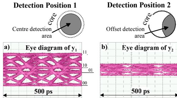
Fig. 2: Eye diagrams of  $y_1(t)$  and  $y_2(t)$  for two co-propagating signals at two different detection position [a)centre detection area; b) offset detection area]
