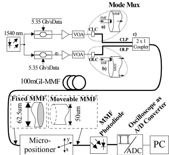
Fig. 1: Experimental setup with two different launched signals (a,b) transmitted over 100m GI-MMF
