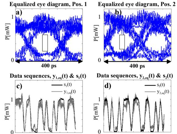
Fig. 3: Equalized eye diagrams for a) detection pos. 1 and b) pos. 2; c,d) comparison of inputs  $s_1(t)$  &  $s_2(t)$  (black) and equalized (grey) outputs  $y_{1,eq}(t)$  &  $y_{2,eq}(t)$
