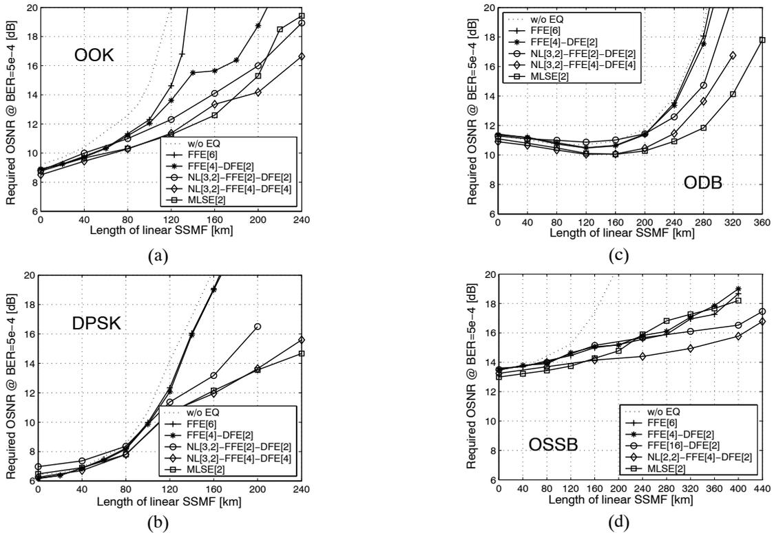
Fig. 2. Required OSNR at  $BER=5 \times 10^{-4}$  versus length of SSMF with and without using equalization for a) OOK, b) DPSK, c) ODB, d) OSSB.
