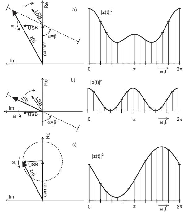
Fig. 1. Phasor diagram, showing upper and lower side bands (USB, LSB) of a single frequency component as well as the carrier and the resulting complex envelope  $z(t)$ . Waveforms with distortions are shown on right hand side. a) OOK, b) ODB and DPSK, c) OSSB. Tip of phasor for  $z(t)$  moves along dotted line in a) b) or circle in c).
