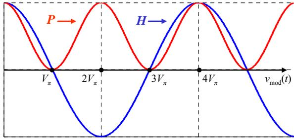
Fig. 3. MZM transfer characteristics.
