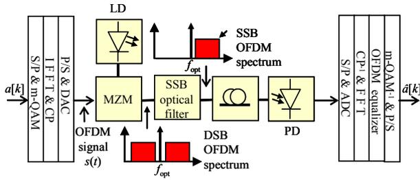
Fig. 5. OOFDM system using IM/DD.
