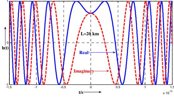
Fig. 4. Impulse response of fiber channel.
