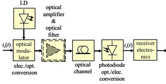
Fig. 1. Block diagram of IM/DD optical system.
