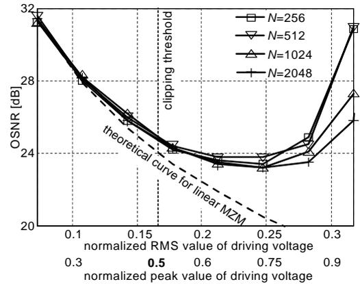
Fig. 8. Required OSNR for  $BER = 10^{-3}$  as function of driving voltage swing.
