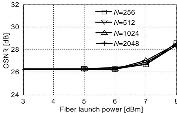
Fig. 9. Required OSNR for  $\text{BER}=10^{-3}$  as function of fiber launch power.
