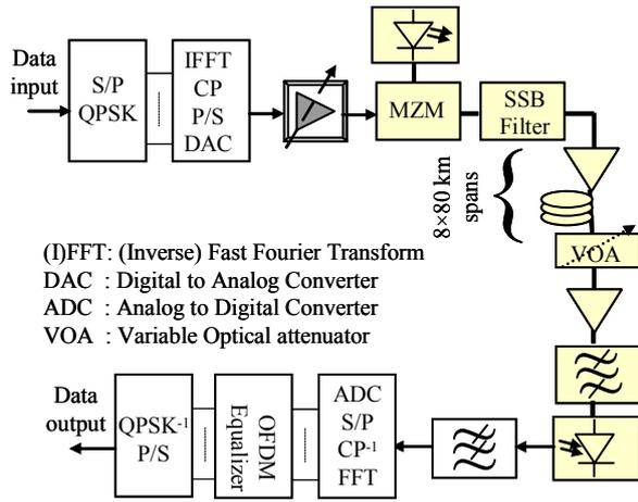
Fig. 7. OOFDM simulation setup.
