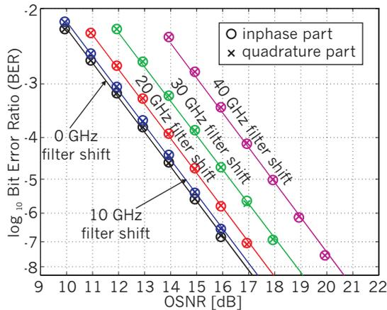
Fig. 2. Simulated BER vs. OSNR for 50 GHz optical filter with 0 GHz, 10 GHz, 20 GHz, 30 GHz and 40 GHz offset from centre frequency.
