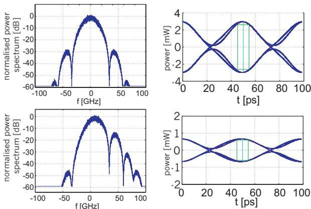
Fig. 3. Normalised PSD (left) and eye diagrams (right) of a 50 GHz Gaussian filtered RZ-DQPSK signal. Top: symmetrically filtered, Bottom asymmetrically filtered with 40 GHz offset from the centre frequency.
