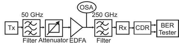
Fig. 1. Simplified block diagram of the experimental RZ-DQPSK setup.
