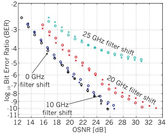
Fig. 4. Measured BER vs. OSNR for 50 GHz optical filter with 0 GHz, 10 GHz, 20 GHz and 25 GHz offset from centre frequency.
