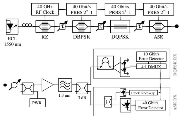
Fig. 1. Block diagram of the RZ-DQPSK-ASK transmitter (top) and receiver (bottom) used in the experiments.
