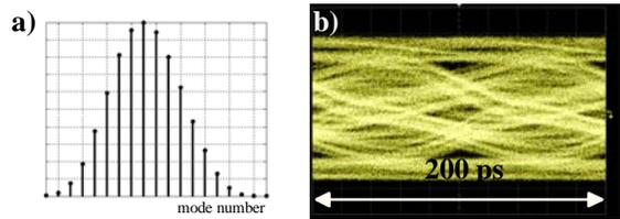
Fig. 3a: Intensity distribution of excited modes for launching with an offset of  $20 \mu\text{m}$  to the core centre; corresponding eye diagram after 200 m MMF
