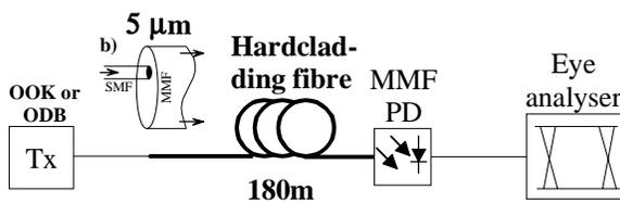
Fig. 4: Two experimental setups with transmitter (OOK or ODB modulation format), launch positions (setup 1:  $20 \mu\text{m}$ ; setup 2:  $5 \mu\text{m}$ ), transmission line (setup 1: 100 m silica multi mode fibre (MMF); setup 2: 180 m hardcladding fibre), multi mode photodiode (MMF PD) and eye analyser
