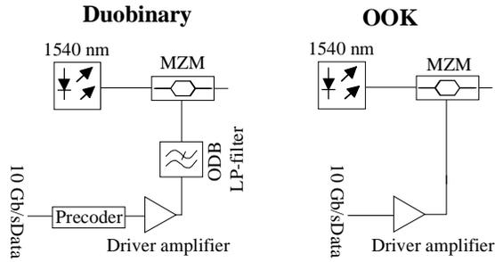
Fig. 5: Transmitter setup for the duobinary (left) and the on-off keying modulation format (right)
