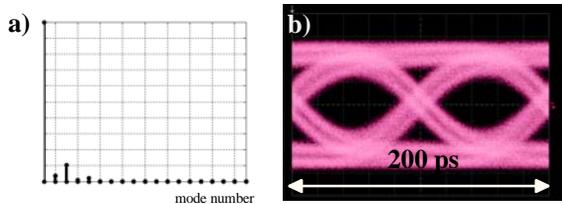
Fig. 2a: Intensity distribution of excited modes for launching at the centre of the core; corresponding eye diagram after 200 m MMF
