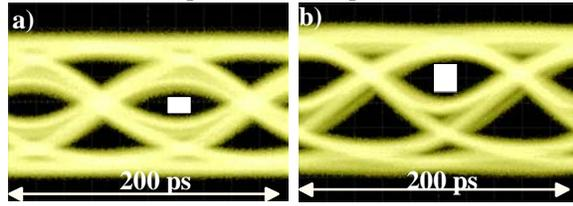
Fig. 7: Eye diagram after 100 m silica MMF using OOK format (left) and duobinary format (right)
