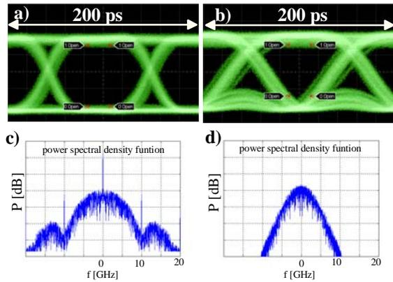
Fig. 6: Eye diagrams for the generated OOK (fig. 6a) and the ODB format (fig. 6b), spectra of the OOK (fig. 6c) and the ODB format (fig. 6d)
