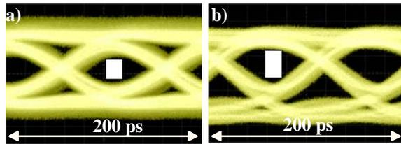
Fig. 8: Eye diagram after 180 m hardcladding fibre using OOK format (left) and duobinary format (right)
