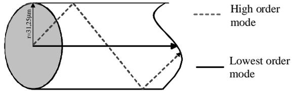
Fig. 1: Schematic sketch of a multi mode fibre (MMF) with the different transmission characteristics of high order modes (dotted grey line) and the lowest order mode (black line)
