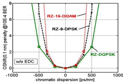
Fig.4: OSNR penalty at BER of  $10^{-4}$  versus CD without EDC for RZ-DQPSK ( $\square$ , solid), RZ-8-DPSK ( $+$ , dashed) and star RZ-16-DQAM ( $\circ$ , dotted).
