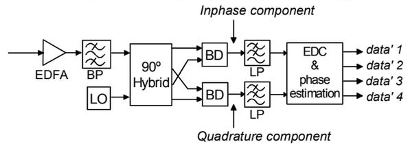
Fig. 3: Coherent receiver setup
