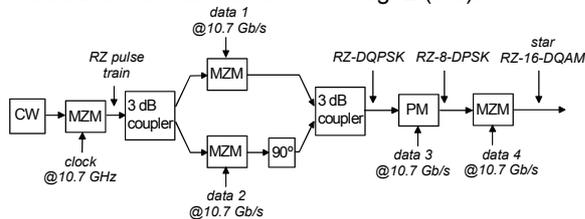
Fig. 1: Transmitter setup; PM: Phase Modulator
