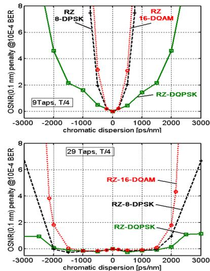
Fig.6: OSNR penalty at BER of  $10^{-4}$  versus CD after equalization with T/4 spacing for a) 9 taps and b) 29 taps. Markers according to fig. 4.
