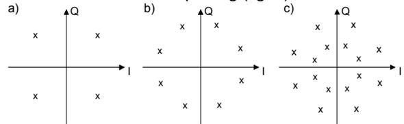
Fig. 2: Signal space constellation of a) RZ-DQPSK b) RZ-8-DPSK and c) star RZ-16-DQAM
