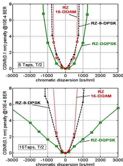
Fig.5: OSNR penalty at BER of  $10^{-4}$  versus CD after equalization with T/2 spacing for a) 5 taps and b) 15 taps. Markers according to fig. 4.
