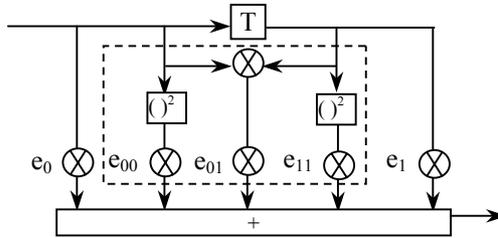
Fig.2. Nonlinear FFE[1]-NL[2]. nonlinear part of setup marked with dash-box.
