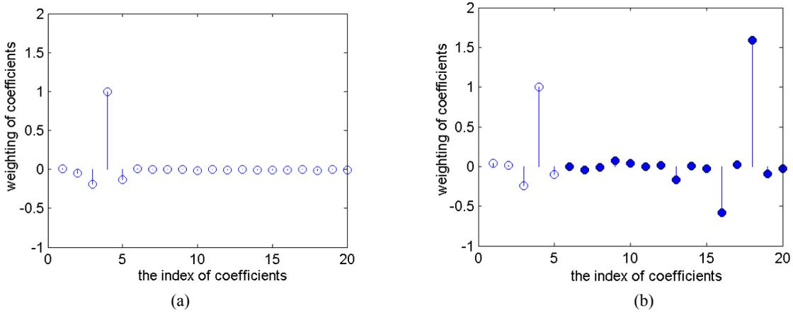
Fig.7. The weighting coefficients of linear FFE[19] (a) and nonlinear FFE[4]-NL[2] (b).
