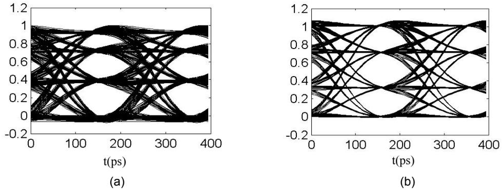
Fig.4. B2b equalized 4-ASK eye-diagrams with FFE[19] (a) and FFE[4]-NL[2] (b).
