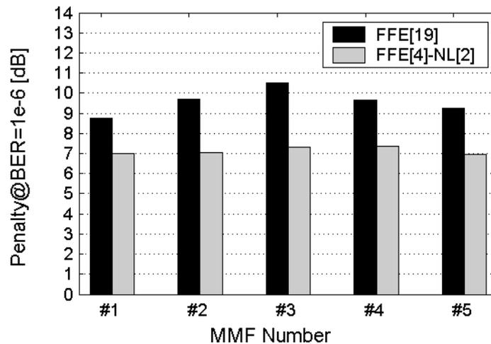
Fig.8. Electrical power penalty compared to b2b for the two kinds of equalizer setups over 300m-MMF for 10Gb/s data rate.
