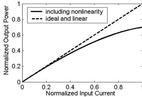
Fig.1. P-I characteristics of linear and nonlinear LD.
