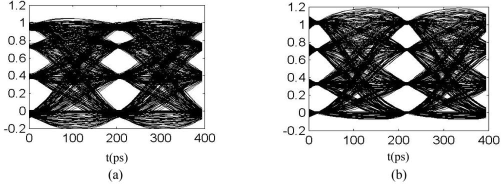
Fig.6. Equalized 4-ASK eye-diagrams over MMF #1 after 300m-transmission distance by using FFE[19] (a) and nonlinear FFE[4]-NL[2] (b).
