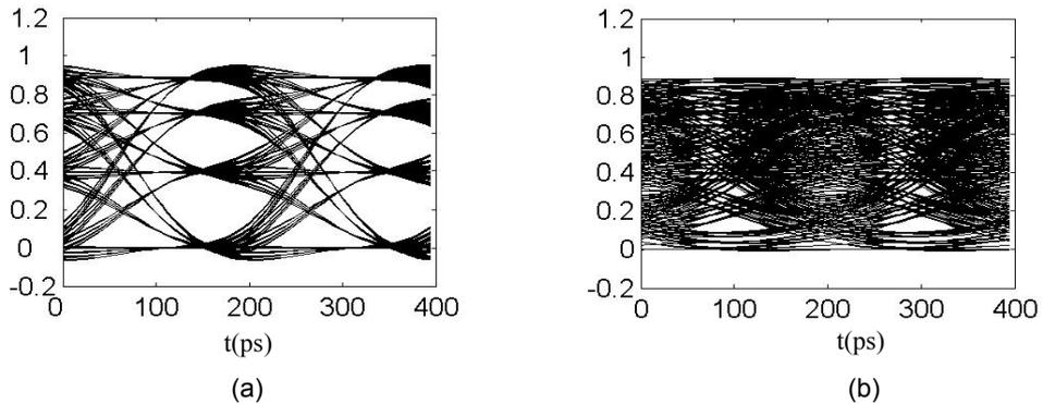
Fig.5. Received 4-ASK eye-diagrams over MMF #1.(a): b2b. (b): 300m-transmission distance.
