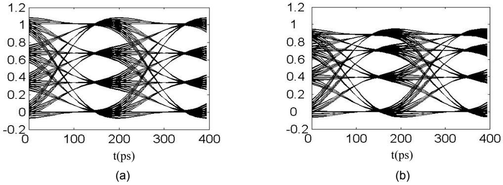
Fig.3. B2b received normalized 4-ASK eye-diagrams with linear (a) and nonlinear LD (b).
