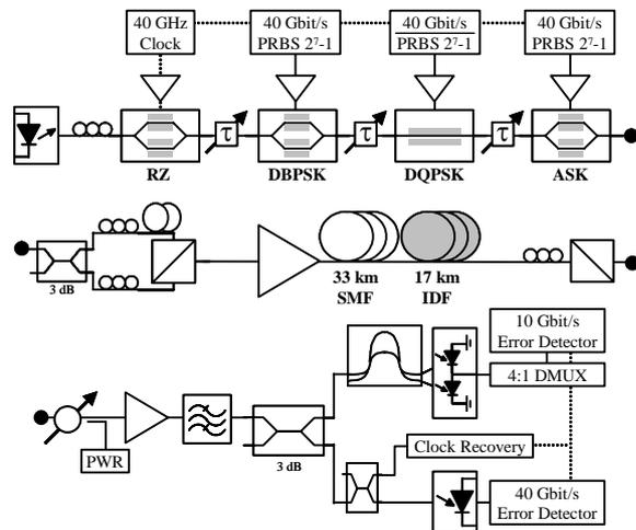
Fig. 1: Simplified experimental setup showing the transmitter (top), transmission span with polarisation multiplexing (middle) and the receiver (bottom).
