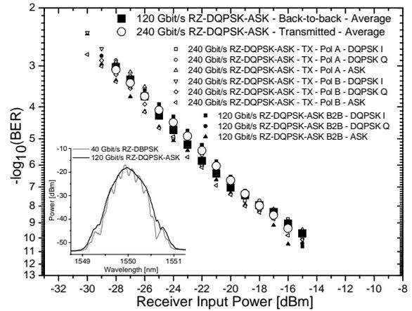
Fig. 3: BER measurements for the back-to-back case and after transmission. The inset shows the optical power spectrum of 40 Gbit/s RZ-DBPSK and 120 Gbit/s RZ-DQPSK-ASK.
