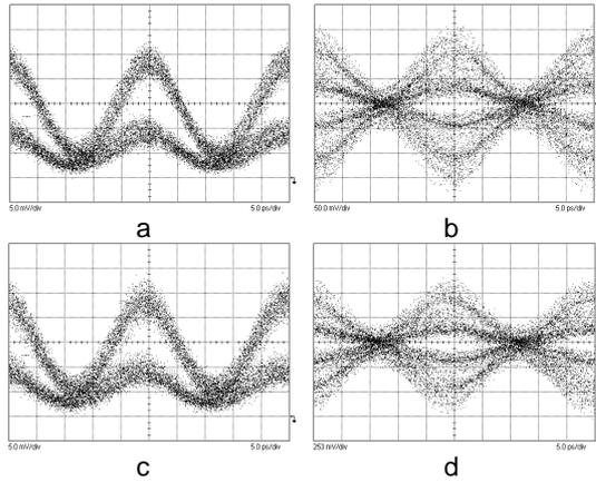
Fig. 2: Eye diagrams of the generated signal (a) and demodulated signal in the back-to-back configuration (b). The received signal after transmission is shown in (c), along with the demodulated signal in (d).
