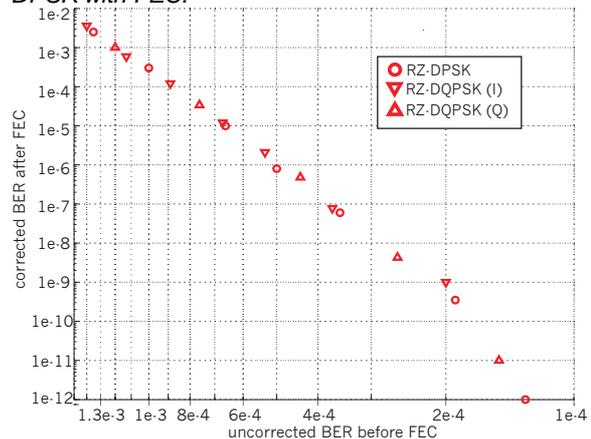
Figure 3: Measured corrected BER after FEC vs. uncorrected BER before FEC for both RZ-DQPSK tributaries and RZ-DPSK, markers according to figure 2.
