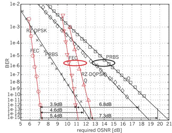
Figure 2: BER vs. required OSNR for both RZ-DQPSK tributaries and RZ-DPSK. Markers:  $\square/\diamond$ : RZ-DQPSK with PRBS  $2^{23}-1$  data;  $\Delta/\nabla$ : RZ-DQPSK with FEC;  $x$ : RZ-DPSK with PRBS  $2^{23}-1$  data;  $o$ : RZ-DPSK with FEC.
