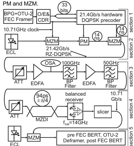
Figure 1: Block diagram of the experimental 21.42 Gb/s FEC encoded RZ-DQPSK transmission set-up.
