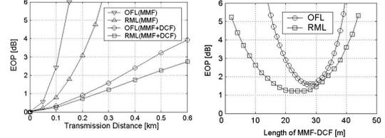
Fig.6: Left: EOP versus transmission distance for OFL as well as RML with and without DCF. MMF( $g < g_{opt}$ , with peak), DCF( $g = 3$ ),  $L_{DCF} : L_{MMF} = 22:300$  for RML,  $L_{DCF} : L_{MMF} = 27:300$  for OFL. Right: EOP versus length of MMF-DCF. MMF( $g < g_{opt}$ , 300m, with peak), DCF( $g = 3$ ).
