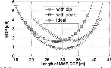
Fig.4: EOP versus the length of MMF-DCF. MMF( $g < g_{opt}$ , 300m), DCF( $g = 3$ ).
