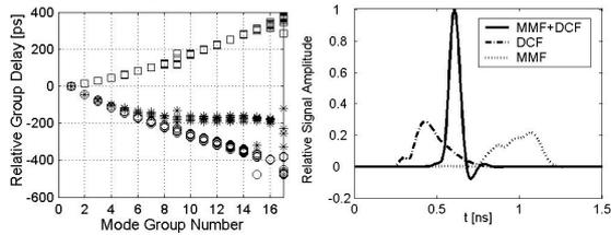
Fig.2: Left: Relative group delay versus mode group number. Square: MMF(300m, ideal), circle: DCF(17m), star: MMF(300m)+DCF(17m). Right: Impulse response of MMF(300m), DCF(17m) and MMF(300m)+DCF(17m).
