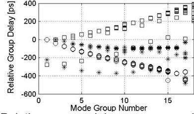
Fig.5: Relative group delay versus mode group number. Square: MMF( $g > g_{opt}$ , 300m, with dip), circle: DCF( $g = 1$ , 16m), star: MMF(300m)+DCF(16m).
