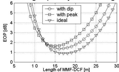
Fig.3: EOP versus the length of MMF-DCF. MMF( $g > g_{opt}$ , 300m), DCF( $g = 1$ ).
