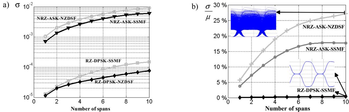
Fig. 4: a) Dependence of standard deviation  $\sigma$  of '1' level towards different number of spans b) Dependence of the ratio  $(\sigma/\mu)$  for different number of spans
