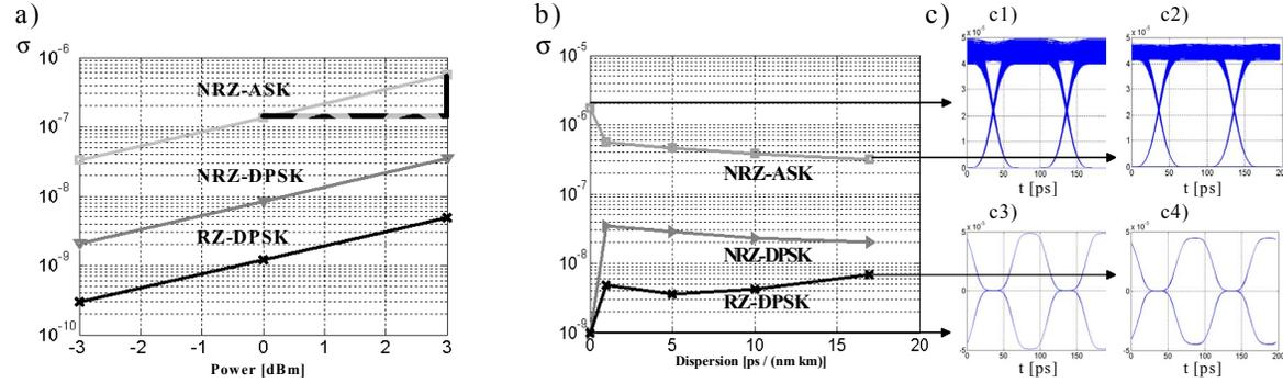
Fig. 3: Dependence of standard deviation  $\sigma$  of '1' level for different modulation formats on a) varying optical power levels b) varying dispersion constants with constant optical power level of 3 dBm after transmission over 100 km; c) eye diagrams for parameter set given in b)
