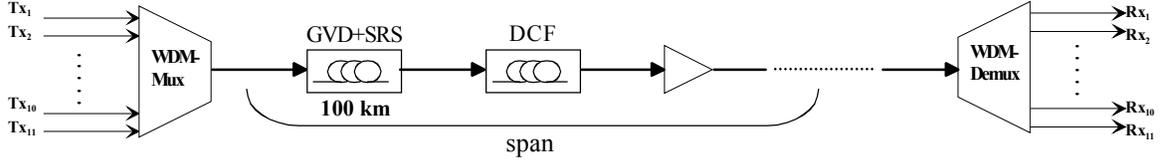
Fig.2: Simulation setup for evaluating the robustness of different modulation formats towards SRS crosstalk
