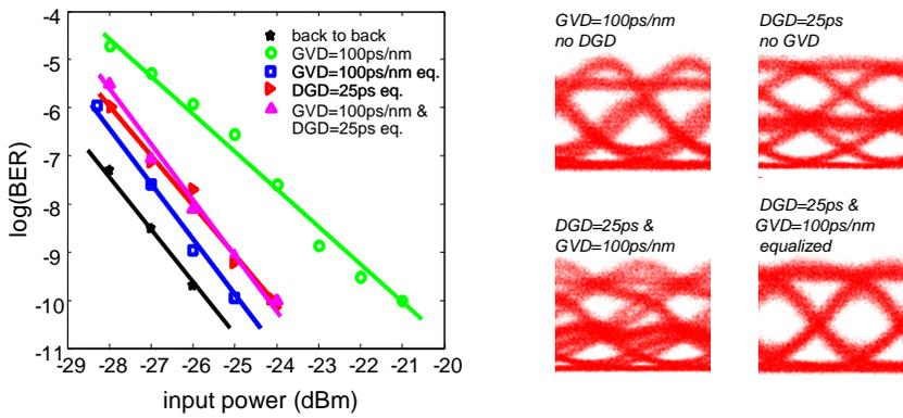
Figure 6. Measurements results of simultaneous CD and PMD compensation: (left) BER, (right) eye pattern diagrams
