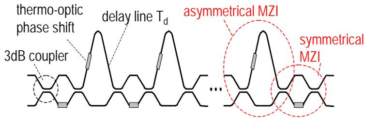
Figure 1. Schematic structure of an integrated optical FIR-lattice filter: cascaded symmetrical and asymmetrical Mach-Zehnder Interferometers (MZI)
