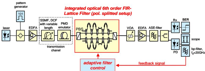
Figure 2. System setup: adaptive equalization with optical FIR-filters and electrical spectrum monitoring. When compensating for PMD, this polarization splitted setup is necessary. Each polarization is equalized with a separate filter. For CD compensation, a single filter without polarization splitting is sufficient.
