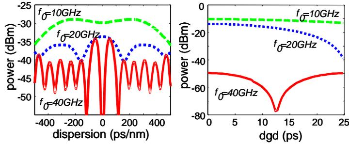
Figure 3. Power response of the received bandpass filtered electrical signal for distortions due to CD (left) and PMD (right) at  $40\text{Gb/s}$
