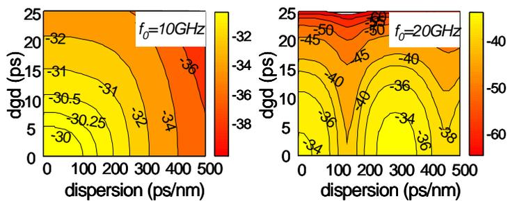
Figure 5. Power response of the received bandpass filtered electrical signal for distortions due to CD and PMD at 40Gb/s: bandpass center frequency  $f_0=10\text{GHz}$  (left),  $f_0=20\text{GHz}$  (right)
