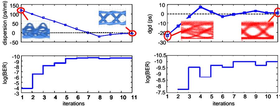
Figure 4. Adaptive compensation results: residual CD of the transmission channel & equalizer, eye patter, BER(left); residual DGD of the transmission channel & equalizer, eye patter, BER(right)
