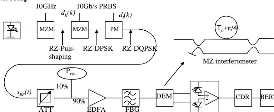
Fig. 1: Experimental setup for RZ-DQPSK at 20Gb/s with autocorrelation detector
