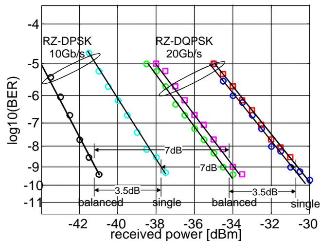
Fig. 2: Measured BER values for RZ-DPSK format at 10Gb/s and RZ-DQPSK at 20Gb/s (real (?) and imaginary (?) component) for balanced and single ended-detection, respectively
