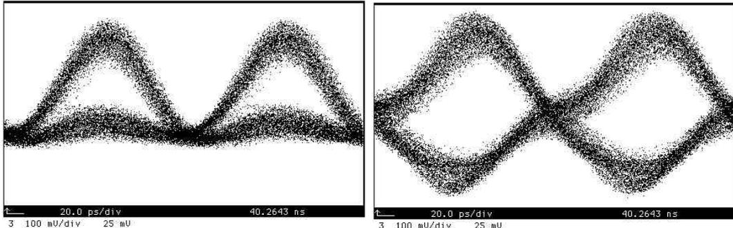
Fig. 3: Measured eye diagrams for imaginary channel of RZ-DQPSK at 20Gb/s for single ended detection (left) and balanced (right)
