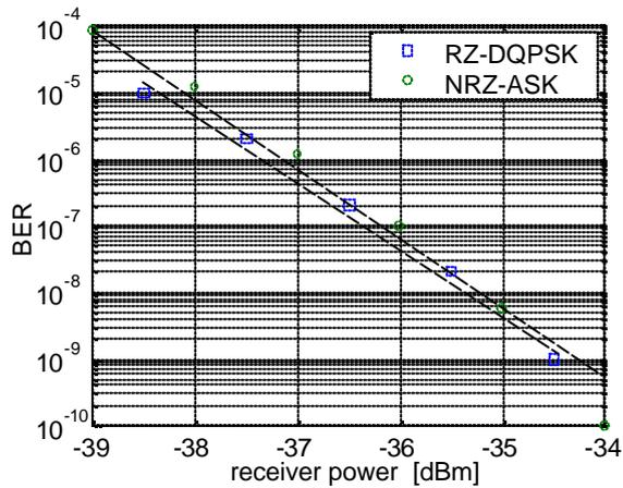
**Fig. 6** Measured BER values for NRZ-ASK format at 10Gb/s and RZ-DQPSK at 20Gb/s, respectively
