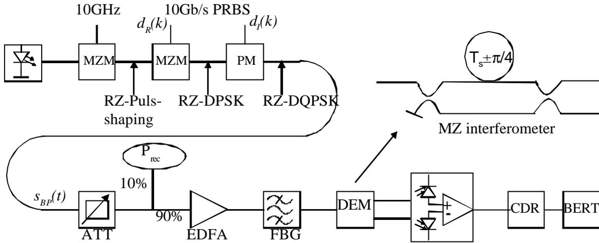
**Fig. 4** Experimental setup for RZ-DQPSK at 20Gb/s with autocorrelation detector
