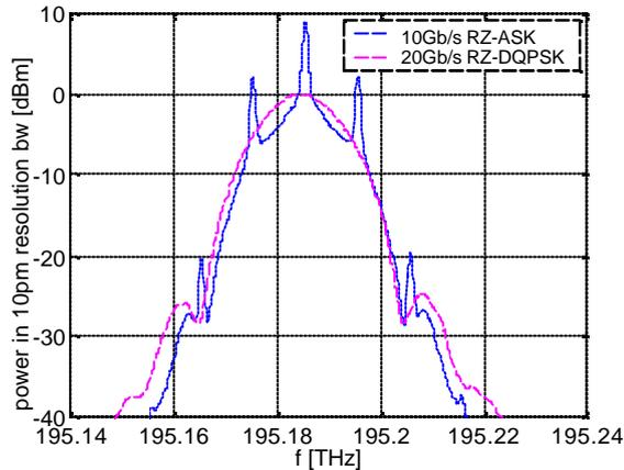
**Fig. 8** Measured data spectrum of RZ-ASK at 10Gb/s and RZ-DQPSK at 20Gb/s
