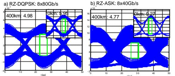
**Fig. 13** Eye opening of a): 80Gb/s-RZ-DQPSK and b): 40Gb/s-RZ-ASK,  $P_{in}=6dBm$ , 400km, 100GHz ch.sp., WDM considering lin. Xtalk, SPM, XPM, FWM
