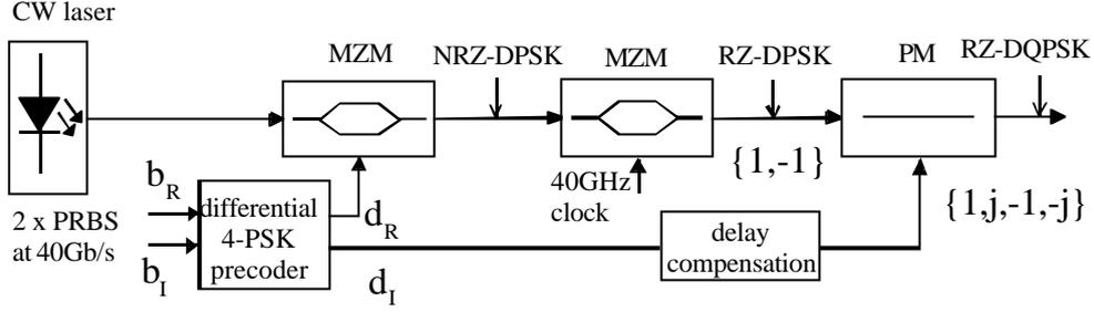
Fig. 1 How to generate an RZ-DQPSK signal
