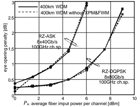
**Fig. 12** Eye opening penalty over  $P_{in}$  for 8x40Gb/s-RZ-ASK, 8x80-Gb/s-RZ-DQPSK: WDM (lin. Xtalk, SPM, XPM, FWM), WDM without XPM&FWM
