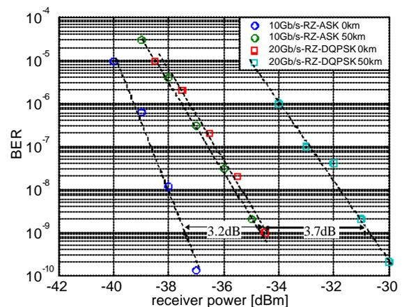
**Fig. 10** Measured BER values versus receiver power for 10Gb/s-RZ-ASK and 20Gb/s RZ-DQPSK after 0 and 50km of SSMF
