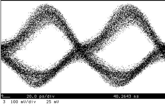
**Fig. 5** Measured eye diagrams for imaginary channel of RZ-DQPSK at 20Gb/s
