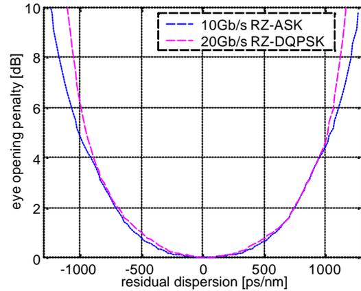
**Fig. 9** Simulated dispersion tolerance of RZ-ASK at 10Gb/s and RZ-DQPSK at 20Gb/s in the linear regime of the fiber
