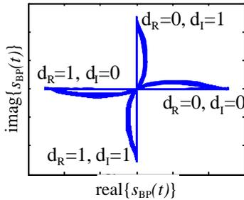
Fig. 2 Trajectories of RZ-DQPSK signal constellation in complex plane
