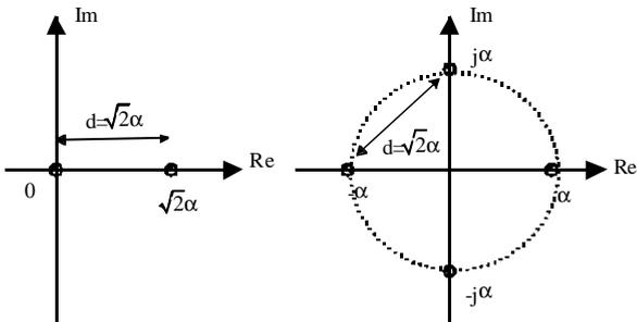
**Fig. 7** ASK (left) and DQPSK (right) in complex plane, for same average power, pulse shape and symbol rate
