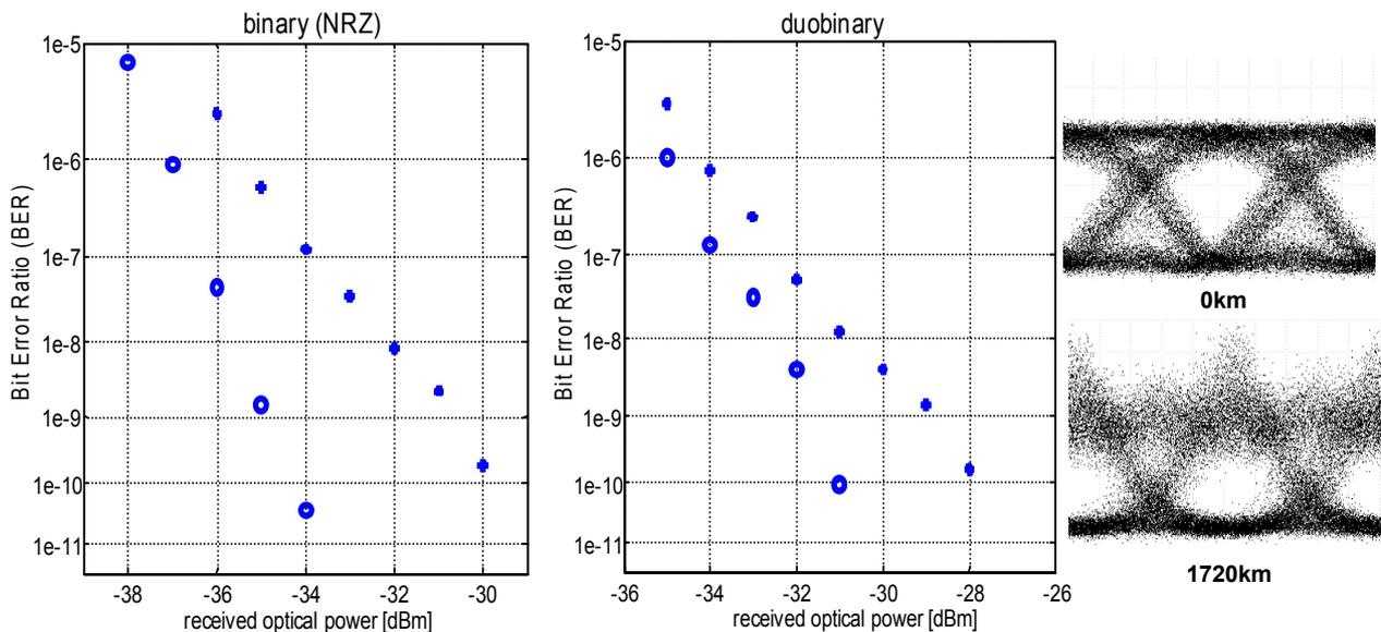
Fig. 3: BER measurements at 10 Gb/s for both modulation formats: standard binary (NRZ) (left) transmission in back-to-back condition (0 km (o)) and after the total link with 1720 km (\*). Measured eye diagrams for duobinary transmission at 0 km and after 1720 km.
