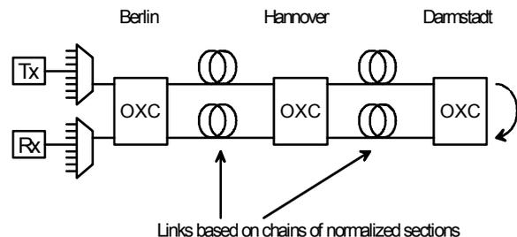
**Fig. 1: System setup of used German - wide WDM network. The signal is looped back transparently at Darmstadt leading to a total link length of 1720 km.**
