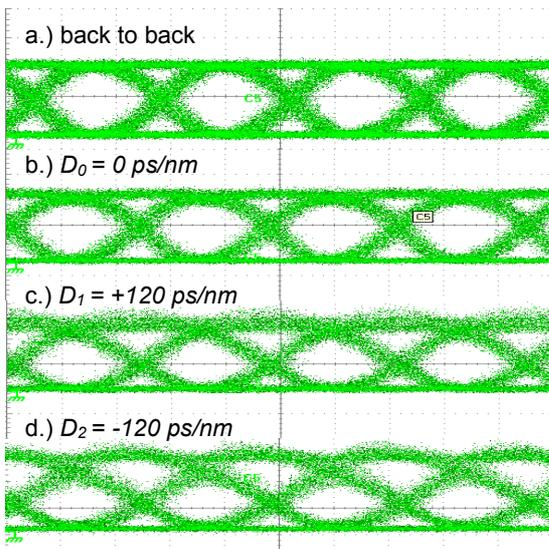
Fig.3: Measured eye pattern @ a.) back to back, compensation of b.)  $D_0 = 0$  ps/nm, c.)  $D_1 = +120$  ps/nm, d.)  $D_2 = -120$  ps/nm
