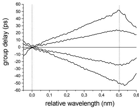
Fig.2: Measured group delay, compensation of dispersion values  $D = +100, +50, -50, -100$  ps/nm
