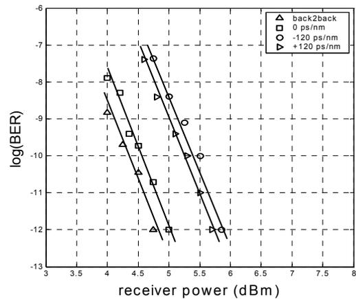
Fig.4: Measured Bit Error Rates @ back to back, compensation of  $D_0 = 0$  ps/nm,  $D_1 = +120$  ps/nm,  $D_2 = -120$  ps/nm
