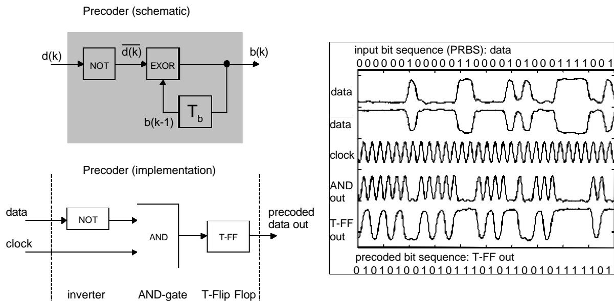
**Figure 5: Schematic of duobinary precoder (left top) and our proposed simple realisation (left bottom) with inverter, AND-gate and T-Flip Flop using standard logic ICs without external feedback. The measured bit sequences at 10 Gb/s (right) after each coding block are shown illustrating the functionality of the proposed precoder.**
