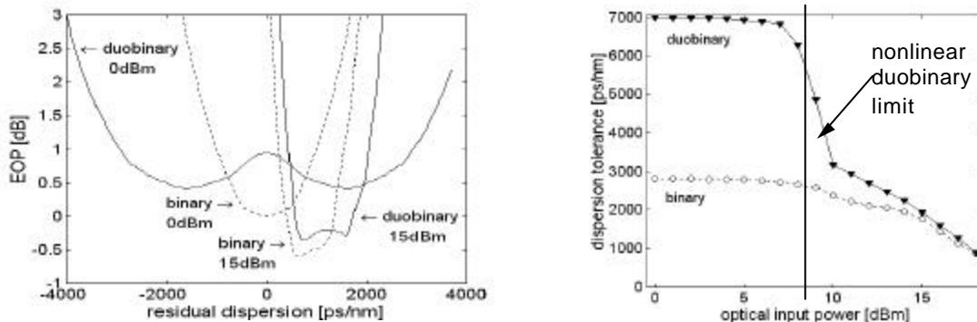
**Figure 4: Comparison of transmission characteristics for binary and duobinary modulation at 10 Gb/s (simulation results): EOP versus residual dispersion for linear (0 dBm) and nonlinear (+15 dBm) transmission (left) and dispersion tolerance ( $Q>10$ ) related to optical input power after 100km SSMF (right).**
