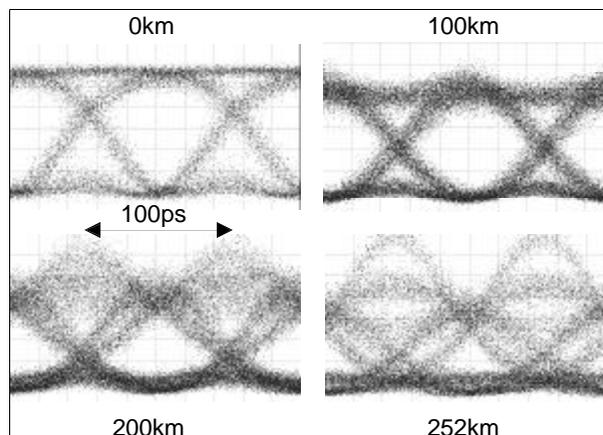
**Figure 7. Eye-diagrams of duobinary transmission at 0km, 100km, 200km and 252km of uncompensated SSMF.**
