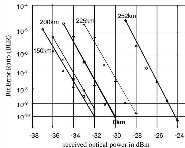
**Figure 8: Measured BER versus receiver input power for 0km, 150km, 200km, 225km and 252km transmission distance over uncompensated SSMF.**
