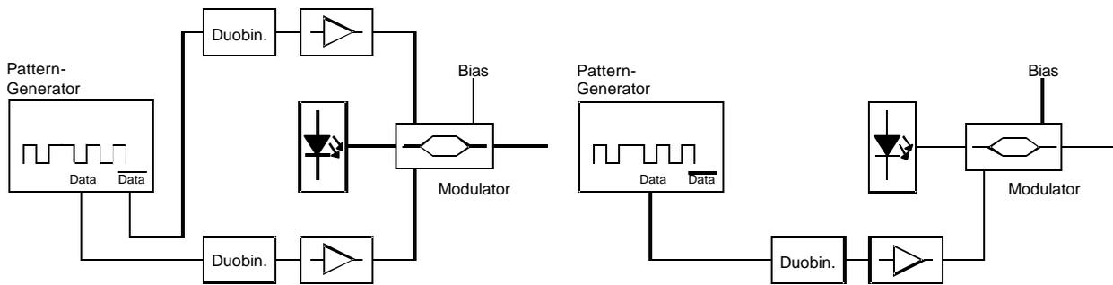
**Figure 6: Conventional duobinary transmitter setup with dual-arm MZM (left) and our proposed transmitter configuration with reduced complexity with a standard single-arm MZM (right).**
