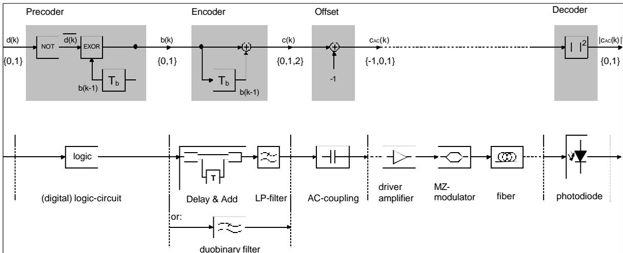
**Figure 1: Overview of duobinary transmission: schematic (top) with precoder, encoder, offset and decoder and possible hardware implementation (bottom) for corresponding functional blocks.**
