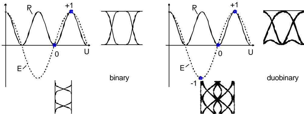
**Figure 2: MZM transfer characteristic of both electrical field (E) and optical power (P) for (conventional) binary modulation (left) and duobinary modulation (right).**
